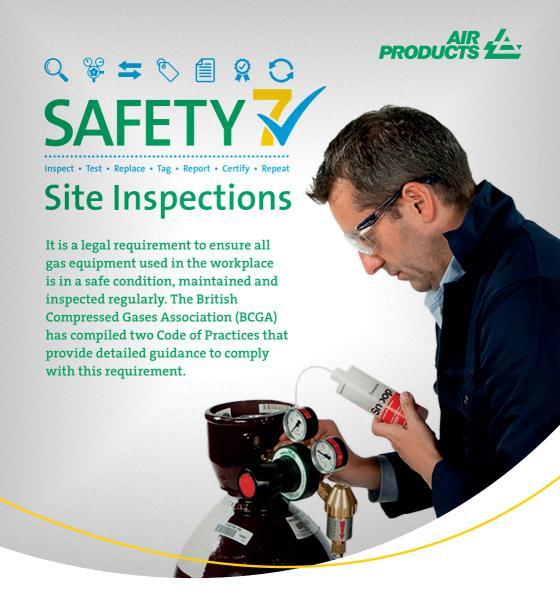
Code of Practice 47 (CP47) details the tests for single cylinder systems, and Code of Practice 7 (CP7) details the testing specifically for oxy-fuel equipment, including regulators and flashback arrestors.
