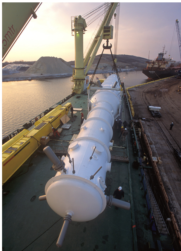
Figure 5. An Air Products CWHE being loaded onto a ship for transport.
