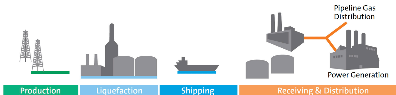
Figure 1. The LNG value chain includes liquefaction of natural gas.
